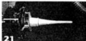
21 Finish-turn the stick, removing the extra length at the tip, then sand.
